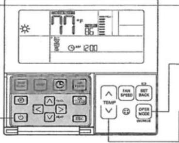
The diagram shows a thermostat control panel with a digital display and various buttons. The display shows a sun icon, a temperature of 77°F, and a battery level indicator. The buttons include a power button, a mode button, a temperature up/down button, a fan speed button, a set back button, and an operation mode button.
